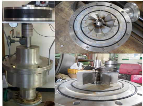
Fig. 9 Photo of power generation system and prototype(4)
