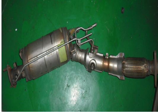
Fig. 1 Picture of commercial DPF used in QM5
