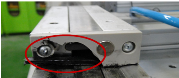
Fig. 4 Failure of transfer plate
