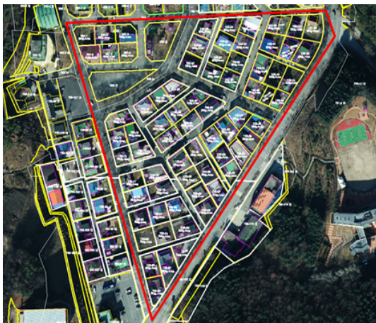
Figure 6. Results Comparison between Cadastral Map (white line) and Stereo Plotting (yellow line) in Case A
