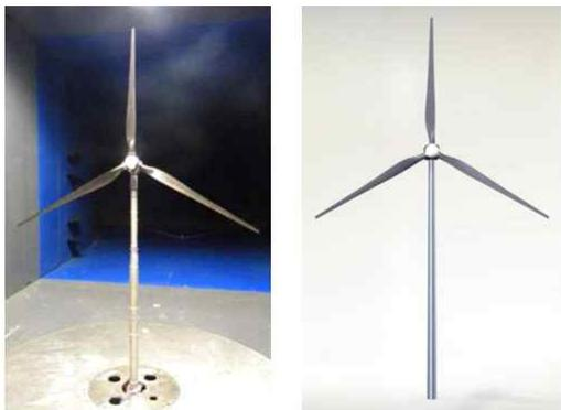
Fig. 1 Scaled Wind turbine: Actual model(left), CAD model(right)
