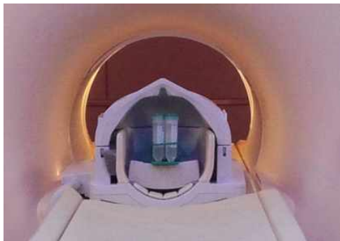
Fig. 1. MRS equipment setting for spectrum measurement.
