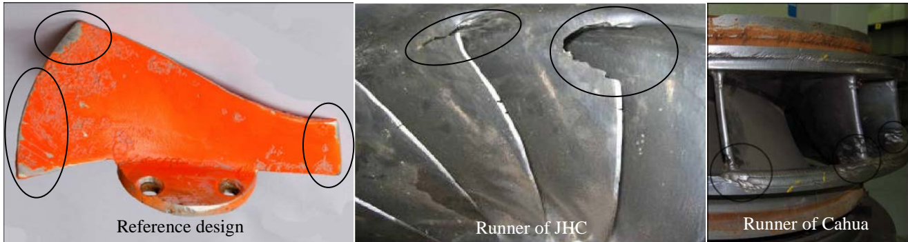
Fig. 5 Wear observed in the test specimen and in the runner outlet of JHC [10] and inlet of Cahua Power Plant [21].
