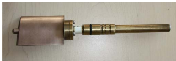
Fig. 1 Model guide vane equipped with instrumented stem
