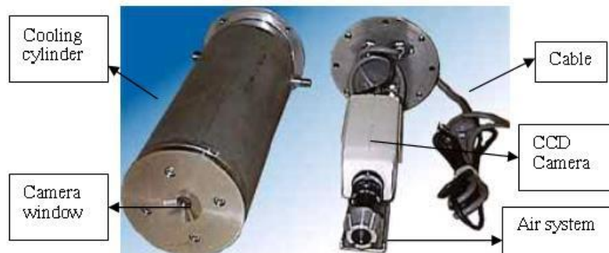
Fig. 1. Components of camera cooling and protecting box: in the camera front, an air system makes the camera lens keep cleaning in a complicated and high temperature environment
