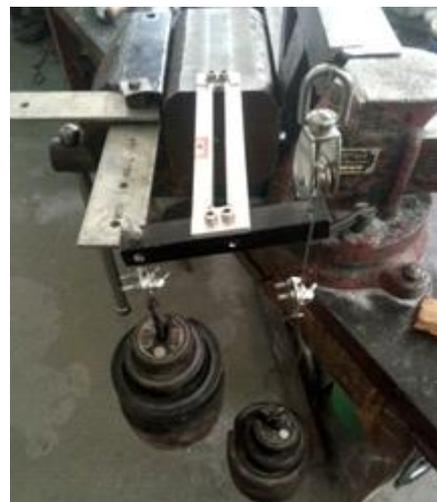
**Fig. 2** Torsional Stiffness Test
