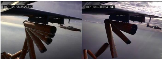
Fig. 8 Flight Test Results of Empty LAU-131 at Inboard (200KCAS (Left) vs 227KCAS (Right))
