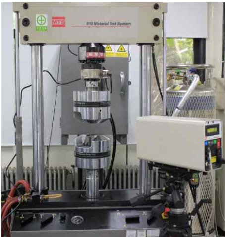
Fig. 7 Tensile Test Equipment with Laser Extensometer
