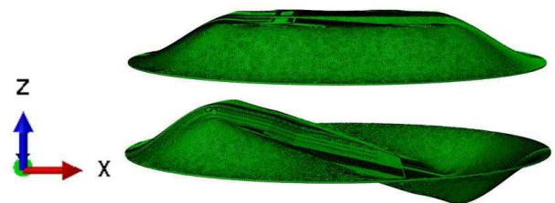
Fig. 8 The 1st, 2ed mode shape of case 1 result
