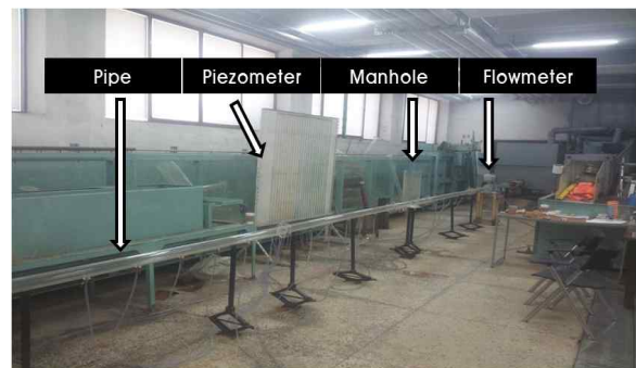
Fig. 2. View of Experimental Apparatus
