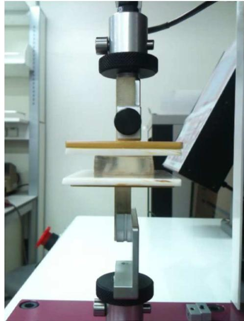
Fig. 2 Expeimetal setup for the unconfined compression of a cylindrical specimen made of gelatin
