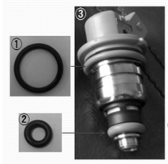
Fig. 4. Replacement of injector O-ring.
