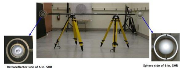
Figure 4 3M ball bar between 2 SMRs (Spherically Mounted Retroreflectors) (Courtesy of NIST)
