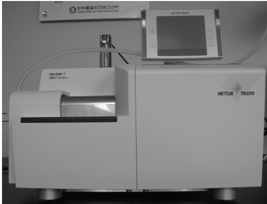
Fig. 2. Thermogravimetric analyzer (TGA/DSC1).
