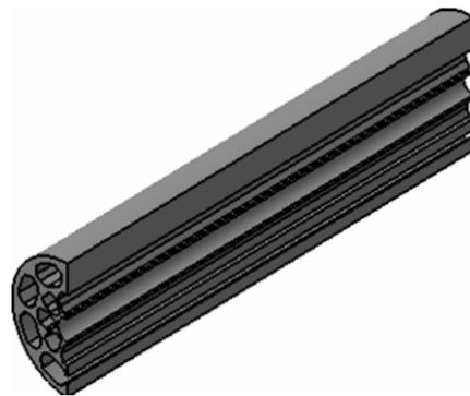
(a) Hollow roller with Y-shaped column
