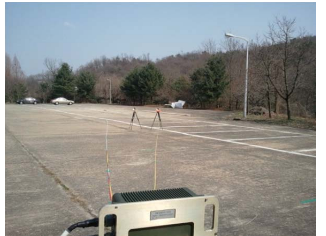
Fig. 9. Photograph of the radar and the corner reflectors.
