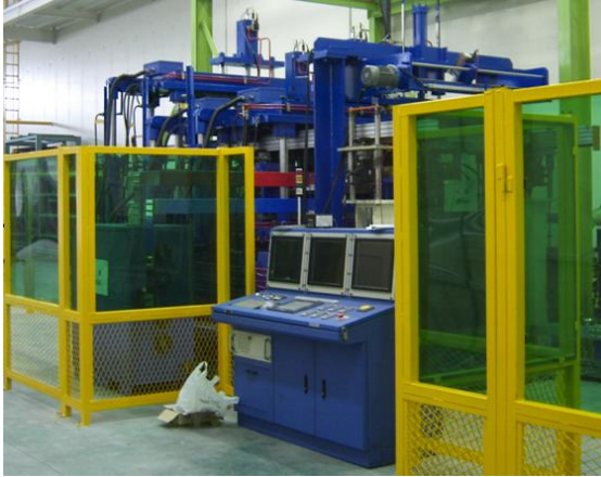
Fig.12 Hot air bulging equipment
