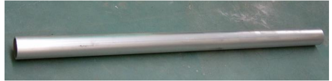
Fig. 1 Seamless pipe of Al5052(diameter 63mm)
