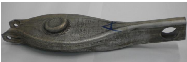
Fig.18 Final product of control arm after wire cutting machining
