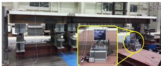
Fig. 5 Experiment setup for acquiring dynamic response of a two-span bridge(El-centro & Kobe)
