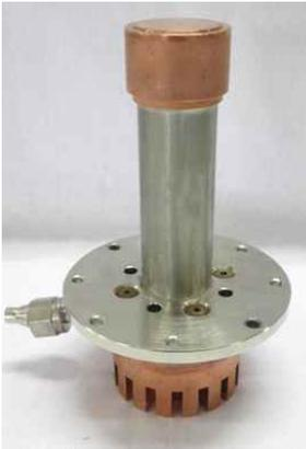
Fig. 5 Fabricated pulse tube expander
