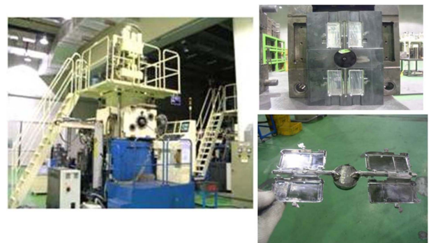
Fig. 3. Photographs of vacuum die casting machine and prepared specimen.
