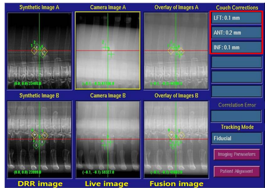
[Fig. 7] Aligning phantom to 3D DOF using two gold markers inserted inside of tumor
