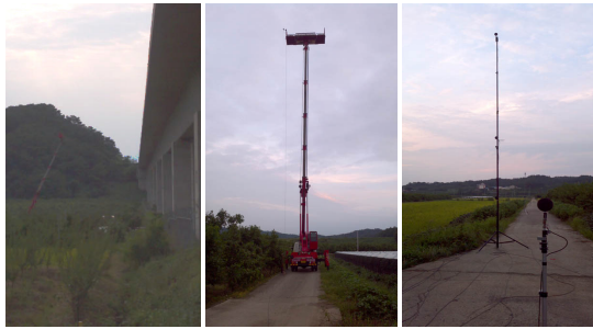
Fig. 4. Measurements of pass-by noise at a concrete bridge.
