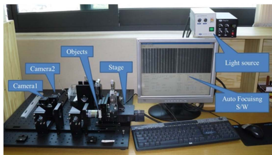
Fig. 1. Focusing experiment set-up.
