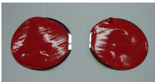
Fig. 1. Epoxy layers separated from wafer substrates.
