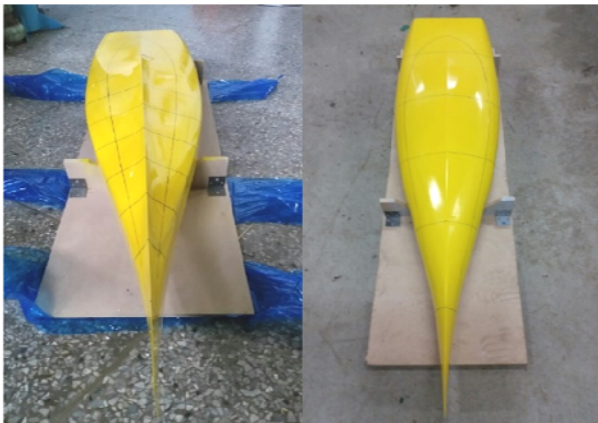
Fig. 1 Figure of wave-piercing V-type and U-type hulls
