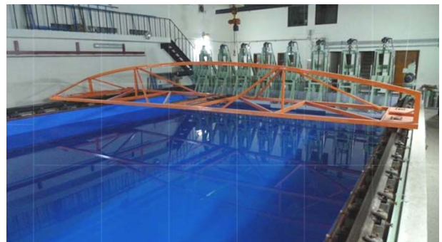
Fig. 5 High speed towing carriage at Seoul National University (SNU)
