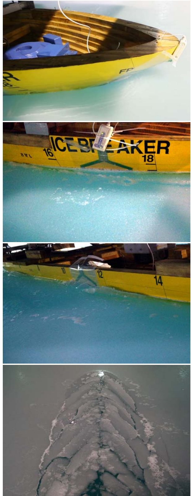
Fig. 7 Icebreaking phenomena and breaking pattern in the model test
