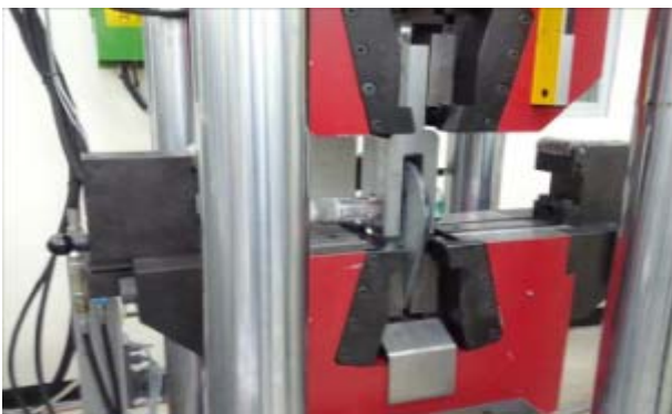
Fig. 2 Test of lug model with UTM
