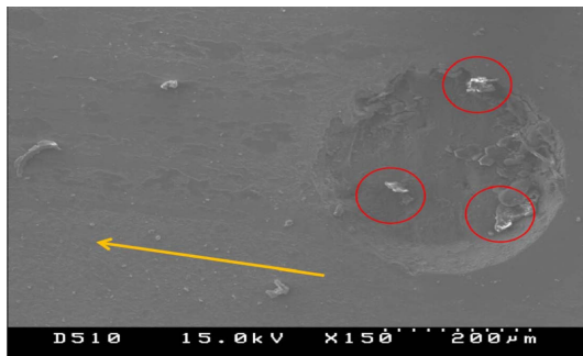
Fig. 8. Wear debris on the dimples after friction test.
