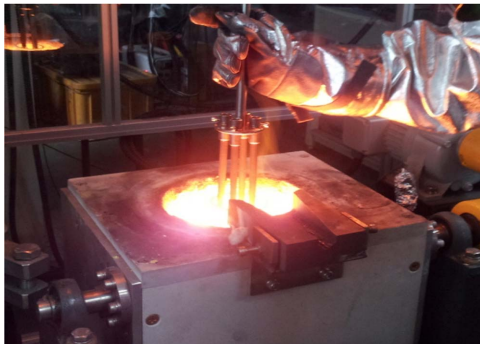
Fig. 1. Slag reforming using carbon rods.
