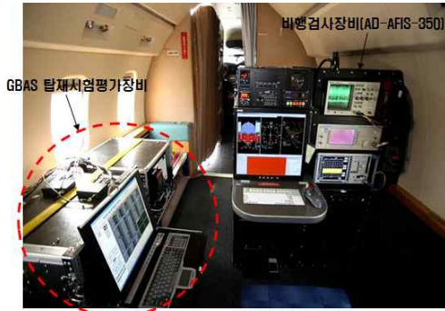
Fig. 8. Flight inspection system and GBAS onboard test equipment
