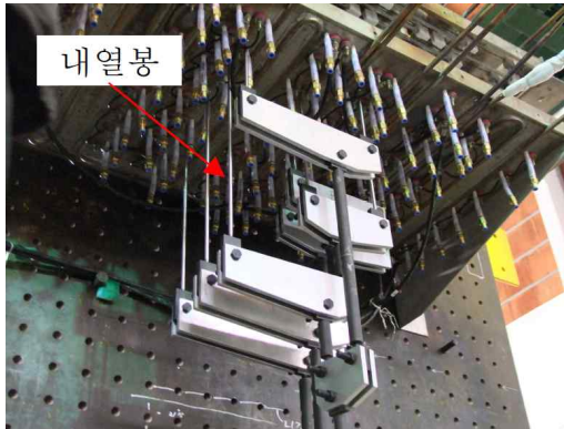
Fig. 5. Whiffle tree and heat-resisting bar of wing testing set
