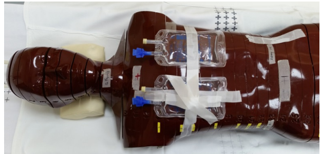
Fig. 2. The RANDO ® phantom, RAN100 represented a 163 cm, 54 kg female figure was used.
