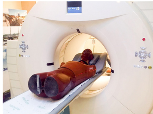
Fig. 3. Anthropomorphic phantom was used for evaluating exposure dose comparison
