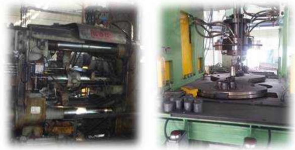
Fig. 1. Horizontal and vertical type of squeeze casting method
