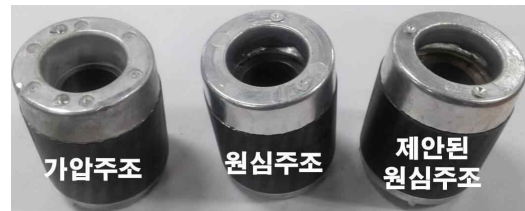
Fig. 4. Manufactured rotor by casting method
