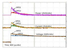
Fig. 8. Typical waveforms of the residual voltages and currents of each SPD in Case 3
