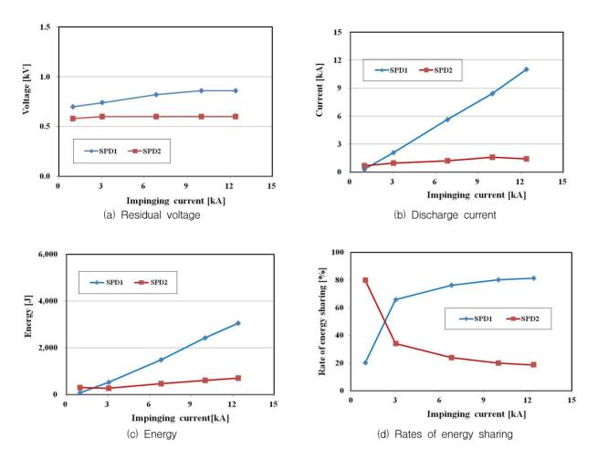
Fig. 9. Measured results of the residual voltages, discharge currents, energy, and sharing rates of each SPD as a function of the impinging current in Case 3
