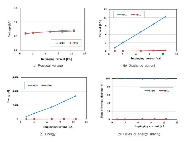
Fig. 5. Measured results of the residual voltages, discharge currents, energy, and sharing rates of each SPD as a function of the impinging current in Case 1
