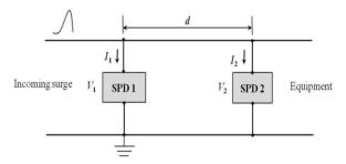
Fig. 1. Cascaded configuration of two parallel connected metal oxide varistors
