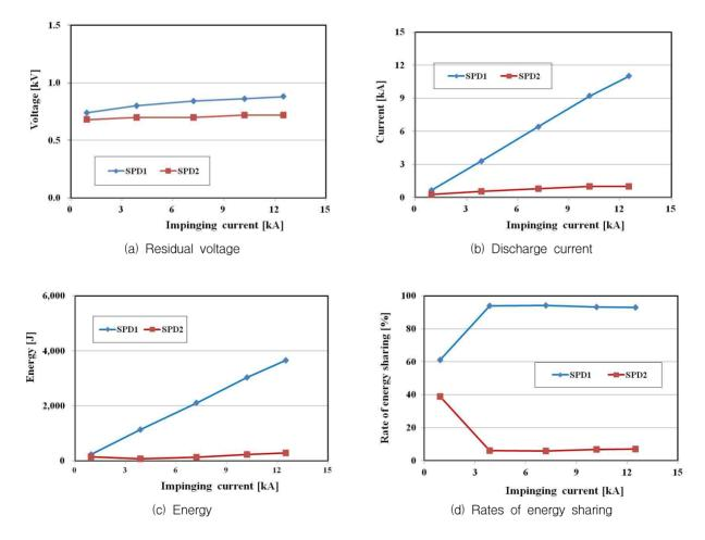
Fig. 7. Measured results of the residual voltages, discharge currents, energy, and sharing rates of each SPD as a function of the impinging current amplitude in Case 2
