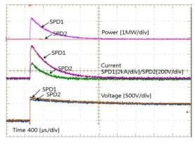
Fig. 4. Typical waveforms of the residual voltages and currents of each SPD in Case 1
