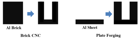
Fig. 2. Comparison between Brick CNC and plate forging
