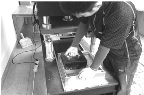
Figure 4. Photographs of the conduct of shear strength test.
