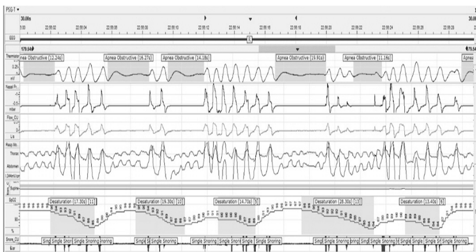
Fig. 4. A sensor for measuring respiratory effort. This record shows the air flow (nasal thermistor and pressure) and respiratory effort measured in the chest and abdomen, and measurements of oxygen saturation (SpO 2 ) and snoring. This record related to obstructive sleep apnea patients indicates that oxygen saturation fell as a result of blocked respiratory flow towards the upper airway.
