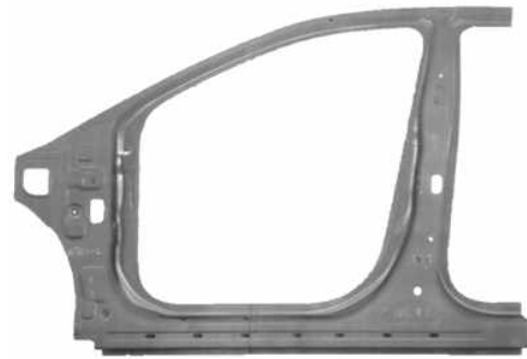
Fig. 16 Final proto type of side structure
