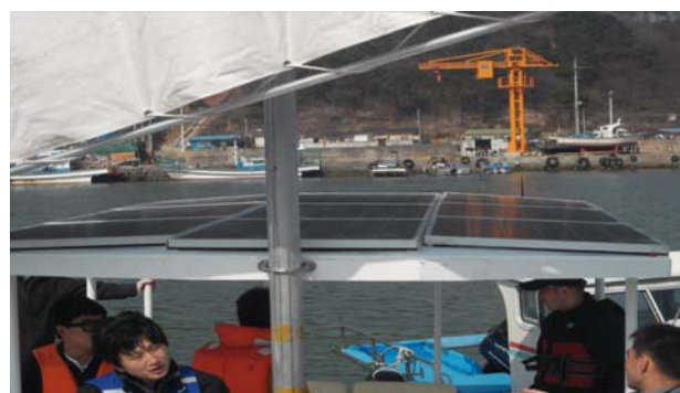
Fig. 6 Modelling image to show the photovoltaic panels used for photovoltaic hybrid generating system
