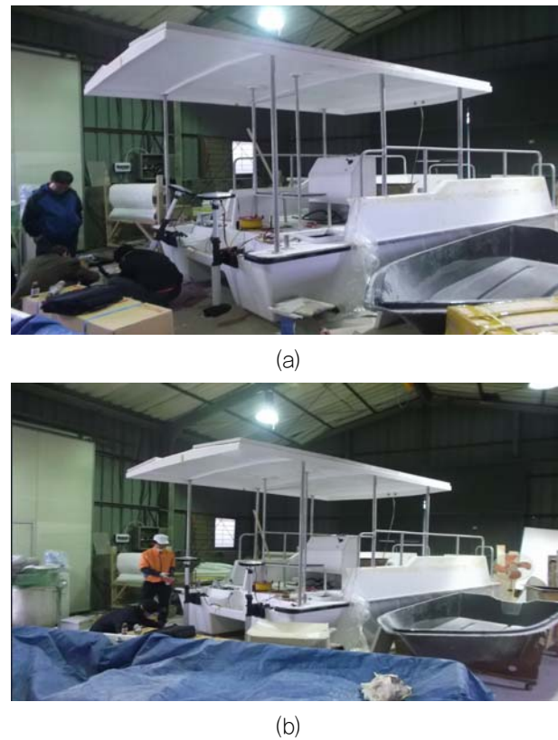
Fig. 9 (a) Image of main frame of leisure ship hull, (b) Image of Internal components leisure ship hull in the process of the fabrication
