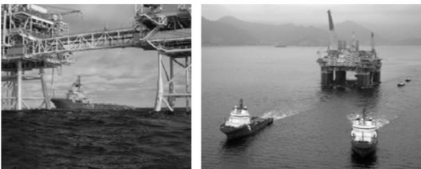
Fig. 1 Examples of OSVs (a platform support vessel and an anchor handling tug supply)
