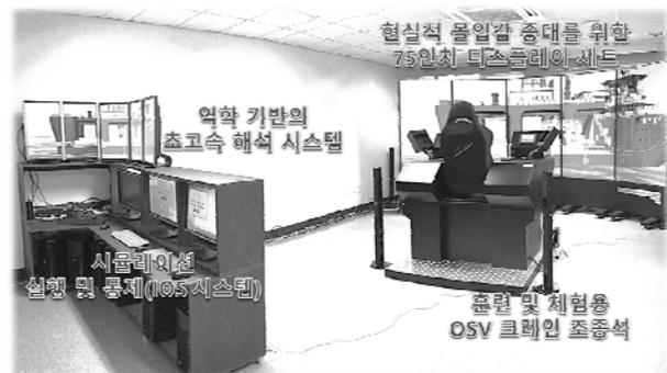
Fig. 6 OSV crane simulator prototype
