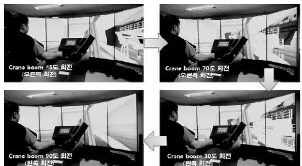
Fig. 12 Procedure of OSV crane turning test
