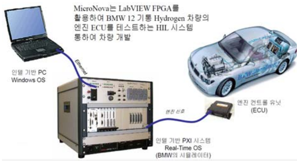
Fig. 7 HIL test system for BMW Hydrogen 7 (Ragonesi et al, 2007)
