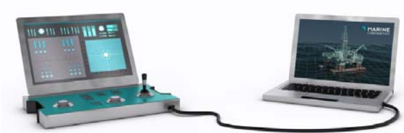
Fig. 9 Drill HIL test for Semi-Rig (Marine cybernetics, 2013)
