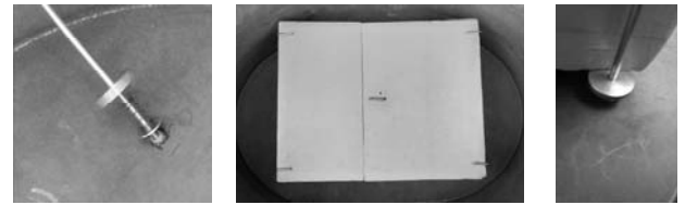
(a) Fixing device (b) Voiding material in the plastic bucket (c) Detail of fixed point
