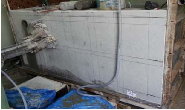
Figure 2. Coring from specimens
