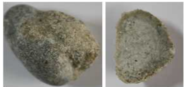
Figure 1. Recycled aggregate and the detached mortar
