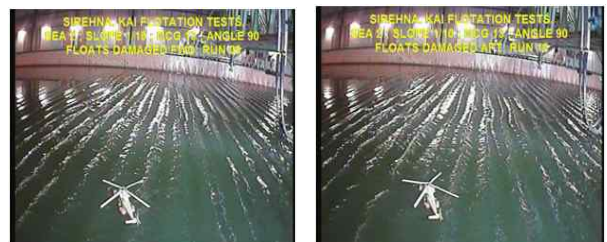
Fig. 11. Floating system test(state #2-puncture)
