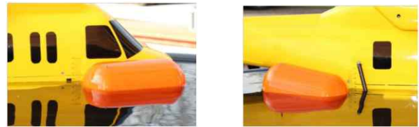
Fig. 5. Waterlines verification using fresh water
