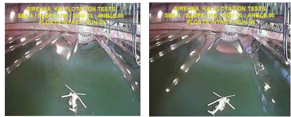
Fig. 10. Floating system test(State #4 - Intact)
